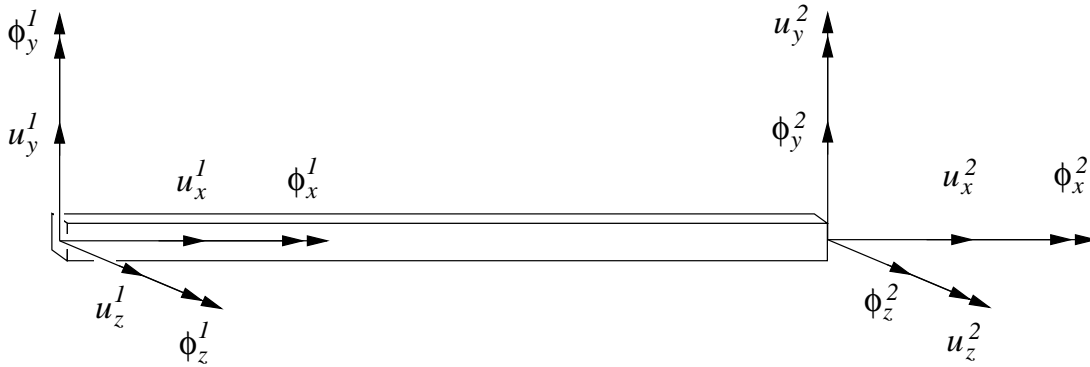
Figure 8.8: Beam element in a local coordinate system with the displacement variables defined.
