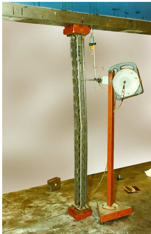
Figure 11: Axial compression of a damaged column.
