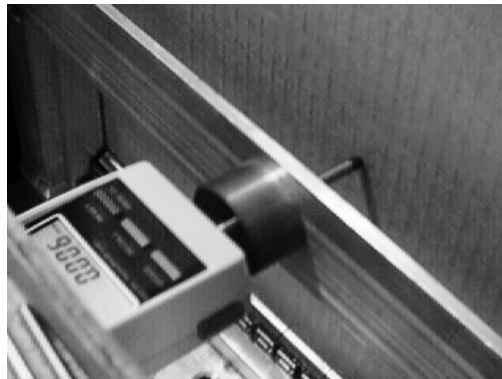
Figure 8. Measuring the deflection of a corrugated panel.
