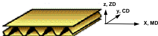
Figure 1. Single-wall corrugated board.
