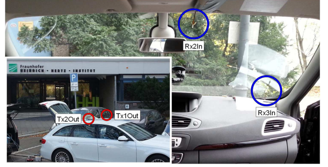
Fig. 1. Position of antennas during measurement: two Tx and three Rx antennas (Rx1Out is in a similar position as Tx2Out).
