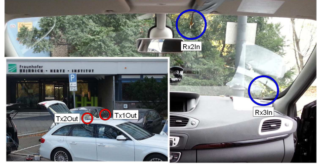
Fig. 1. Position of antennas during measurement: two Tx and three Rx antennas (Rx1Out is in a similar position as Tx2Out).
