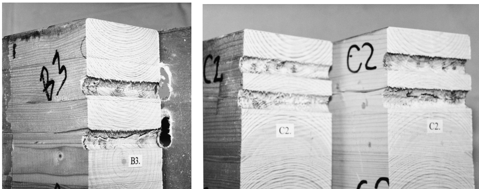
Figure 7 Series B and C, typical failures of glass fibre reinforced specimens. The holes are elongated (3-5mm) and only curved corresponding to the elastic deformation of the dowels.
