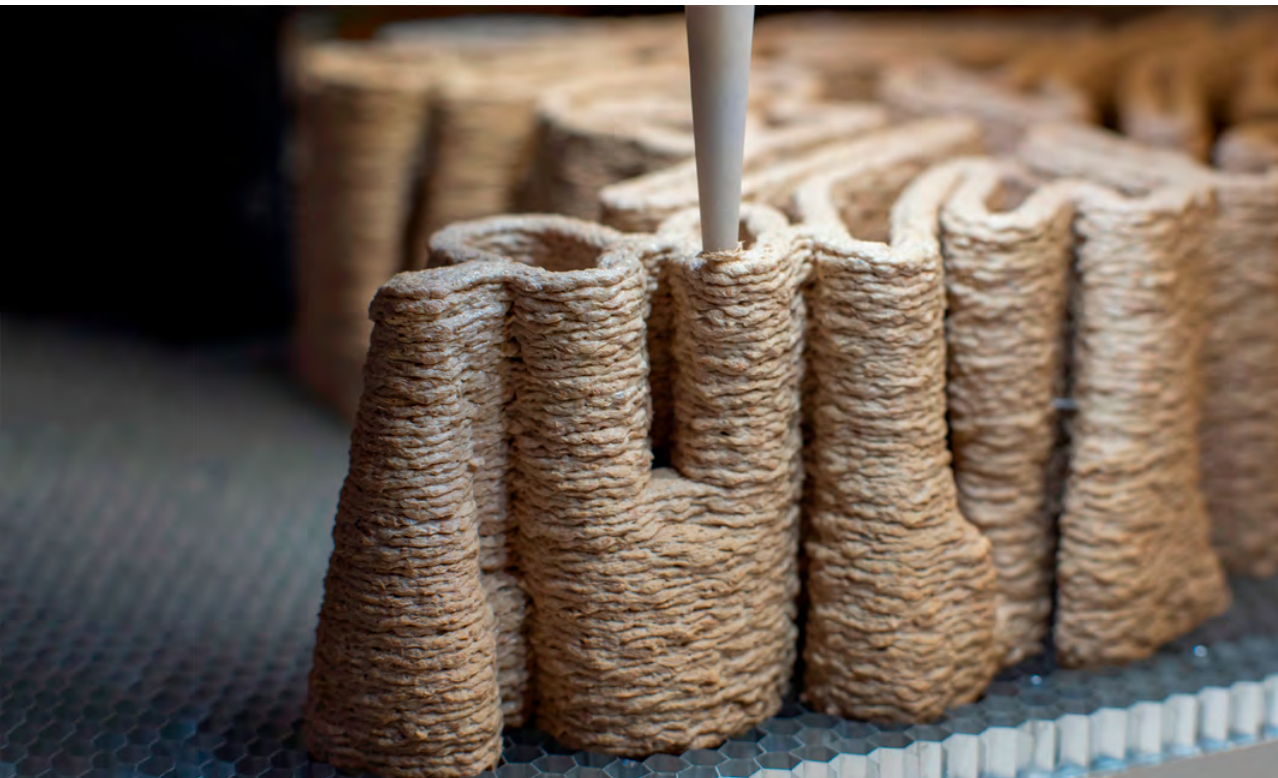
Fig. 7. 3d printing with living pulp.
