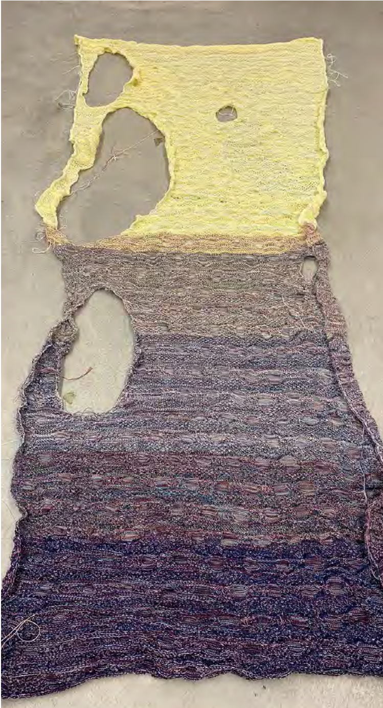
The result of the 3d CNC knit, that accounts for the curvature of the wall and ridge protrusion.
