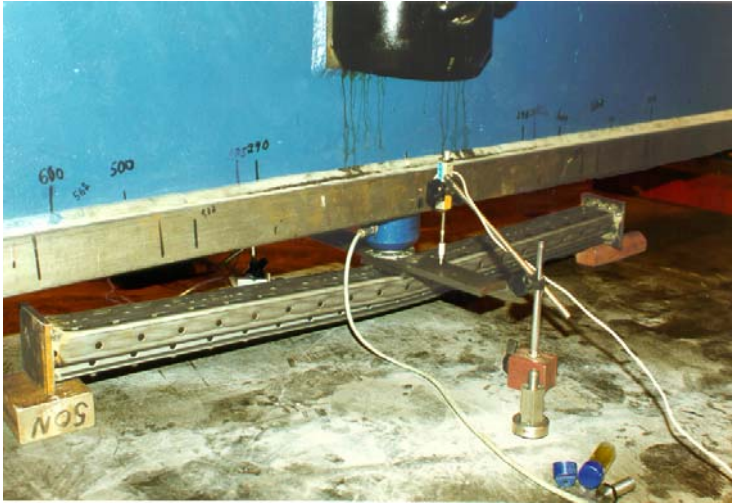
Fig. 10. Compression of a steel bar to the broad side of a column.
