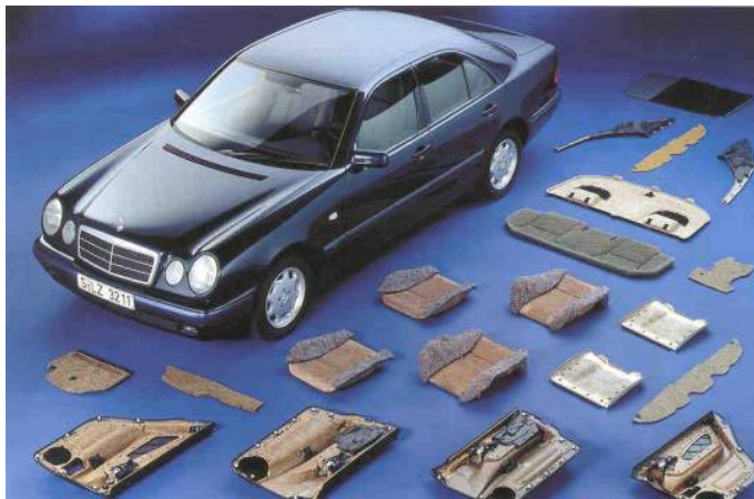
Figure 1. Mercedes E-class showing interior parts of natural fibres [1].
