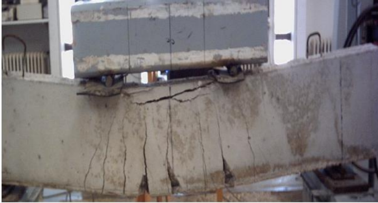
Fig. 12. Flexural failure for control beam.
