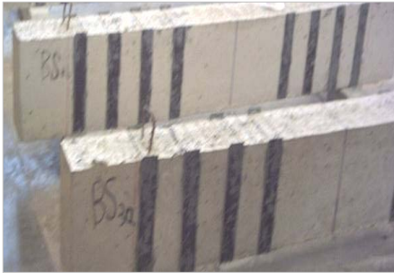
Figure 3. Installation CFRP in experimental work.
