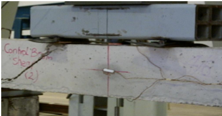
Fig. 17. Shear failure for control beam.
