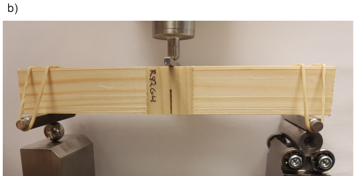
Figure 3: Test-setup and geometry for the fracture energy test (a), where the SENB-specimen was simply supported and loaded in three-point bending (b).
