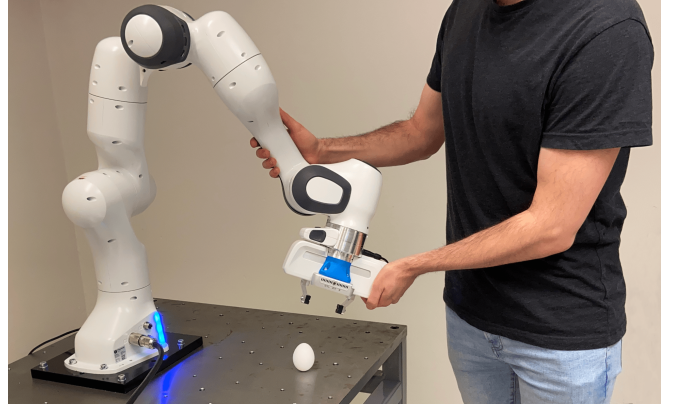
Fig. 1. Setup for the kinesthetic teaching task described in Sec. IV-B. A Franka Emika Panda robot is mounted on a table. The blue piece allows to attach a camera to the robot's end effector. The human operator is manually guiding the robot and displacing it away from its original trajectory and arbitrarily close to the object of interest, here, an egg.
