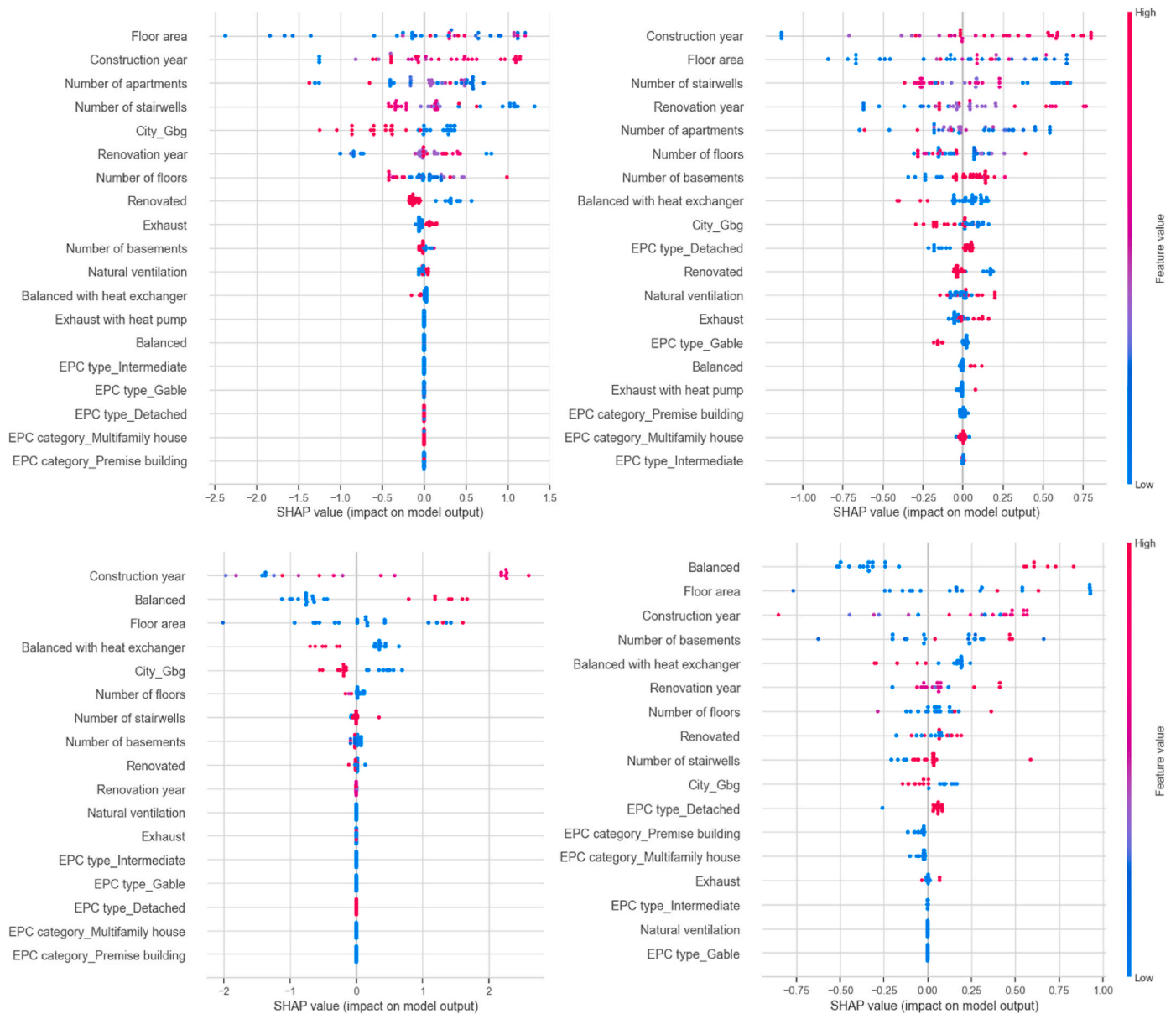
Fig. 8. The summary plots visualize the impact of features on the model output. The observations were represented as a single dot for each feature and densified along the x-axis. The red dots in the feature flow signified high feature values, while the blue dots were low feature values.
