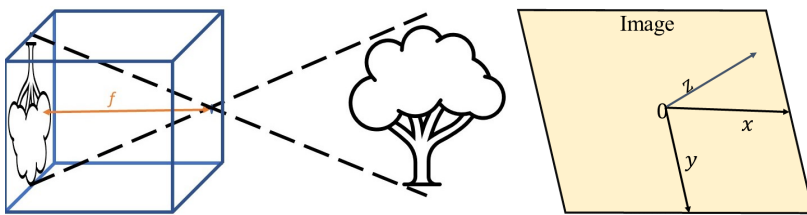
Figure 6.1: To the left: As light rays pass a small aperture they create an image of the world on the back of the camera. The distance from the aperture to the image is known as the focal length denoted by f . To the right: The camera's coordinate system in an image, where Z points outwards.
