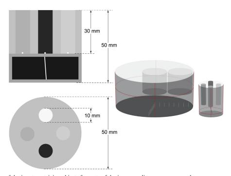
Fig. 3. Drawing of the insert containing objects for parts of the image quality assurance procedures.
