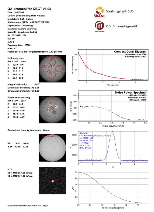
Fig. 7. Software-generated PDF protocol of image quality assurance results.
