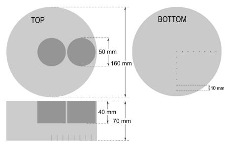
Fig. 2. Drawing of the main body of the phantom.
