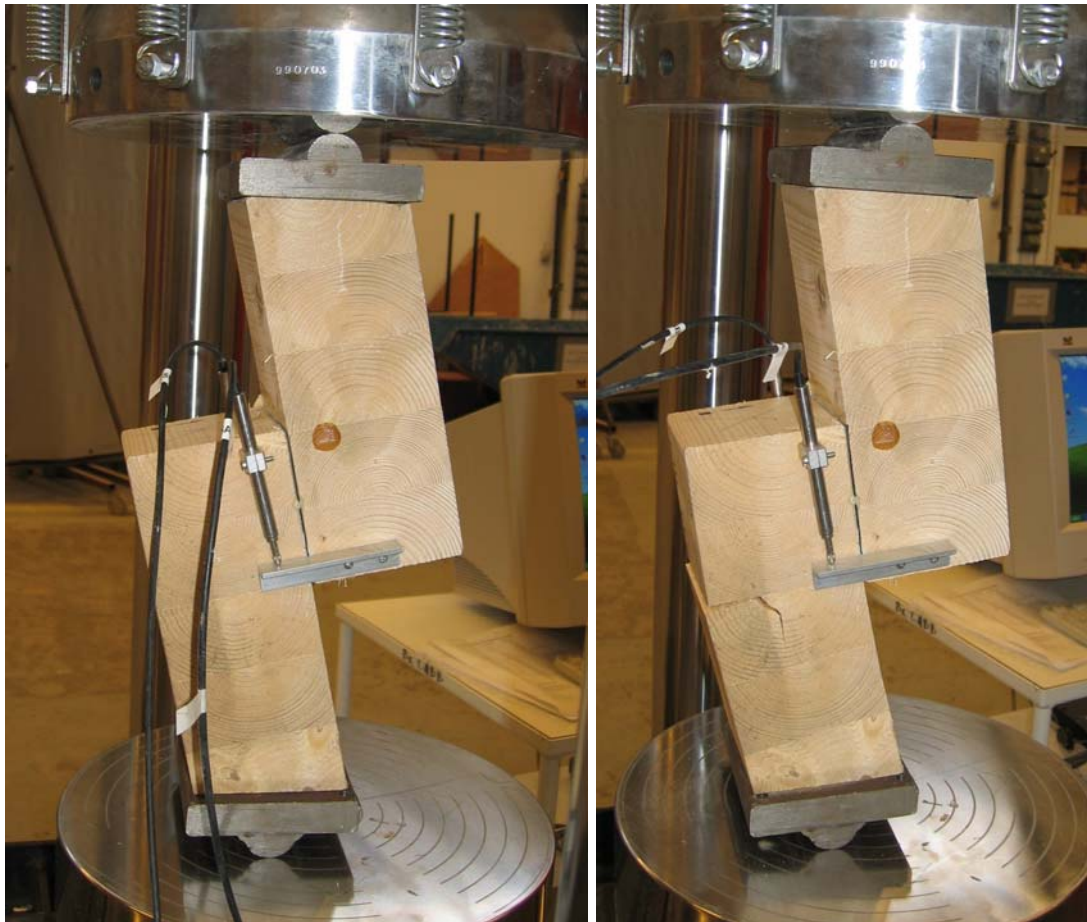
Series 2, rolling shear
