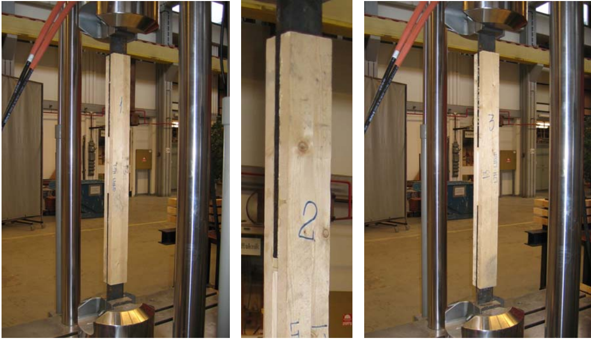
Series 13, inner steel plate rubber foil lap joints, 320 mm
