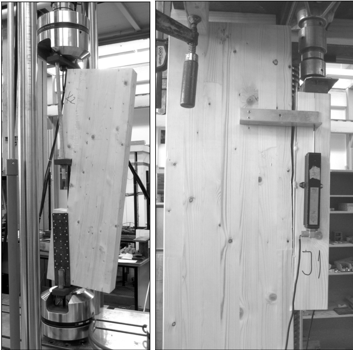
Figure 11. Test setup for test series k (left) and upper support in series j and s (right).
