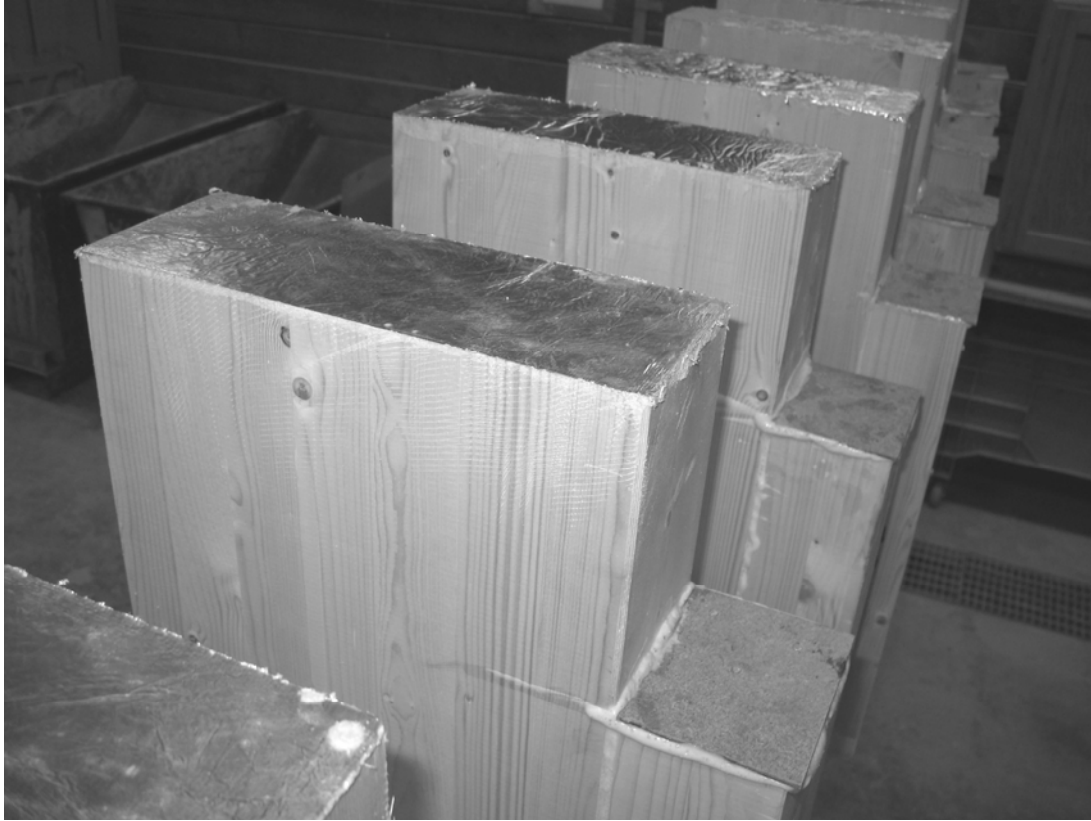
Figure14. End grain sealing of specimens in series o and p.
