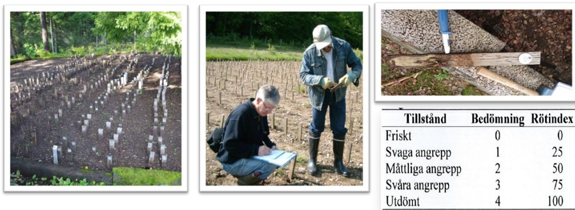
Figure 14. Field test according to EN 252.
