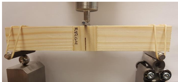
Figure 26. Three-point SENB specimen used for determination of specific fracture energy.
