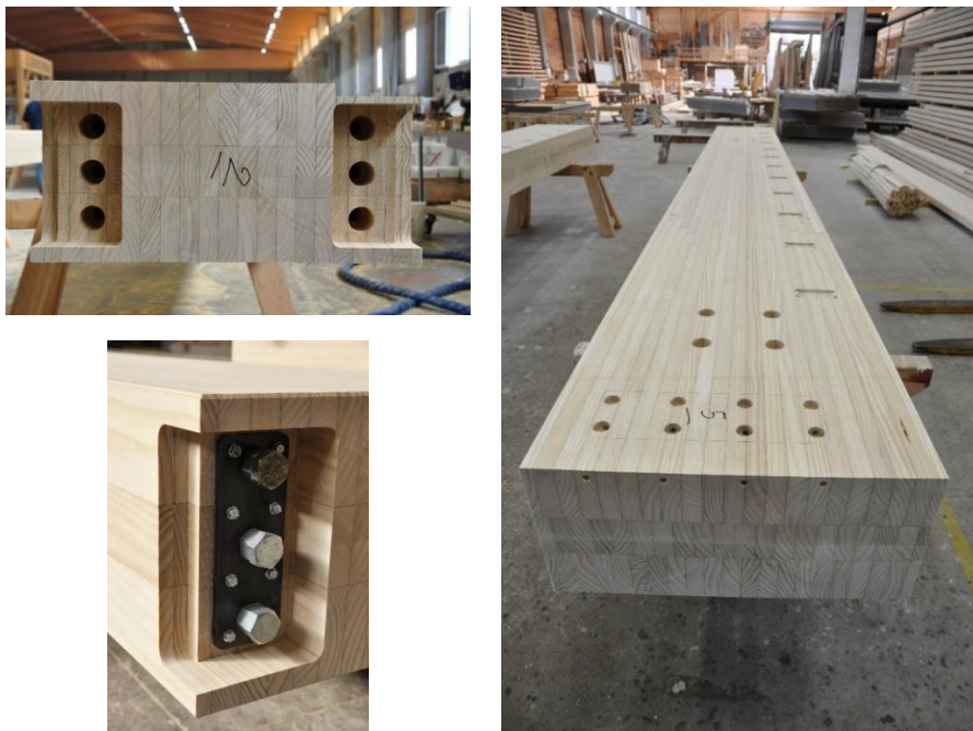
Figure 36. Manufacturing of glued-in rod connections at partner Simonin.
