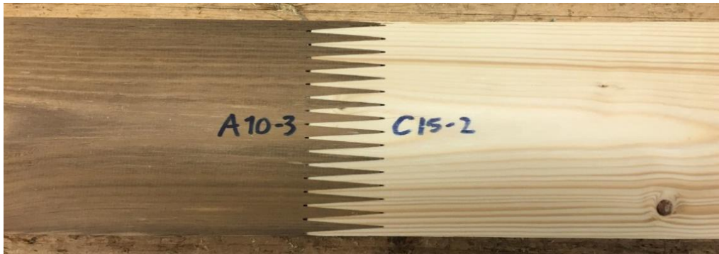
Figure 30. Finger-joint of (left) acetylated juvenile pine (AJP) and (right) untreated spruce (US).
