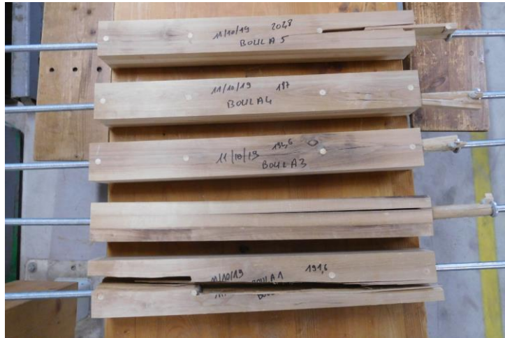
Figure 40. Failure mode for acetylated Birch samples.
