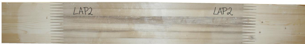
Figure 31. Center section of a glulam hybrid of acetylated birch (mid part) and untreated spruce (outer parts)
