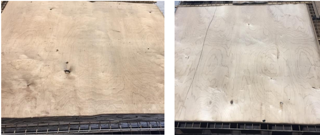
Figure 10. Acetylated birch veneers.
