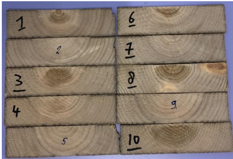
Figure 5. Slices of acetylated scots pine showing heartwood, sapwood, checking and “burning spots”.
