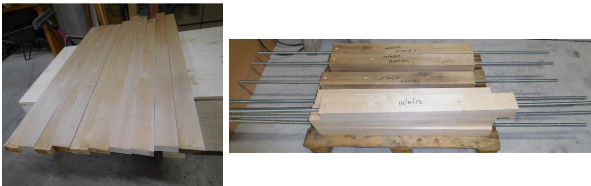
Figure 38. Solid birch (left) was used to manufacture specimens for testing of glued-in rods (right).
