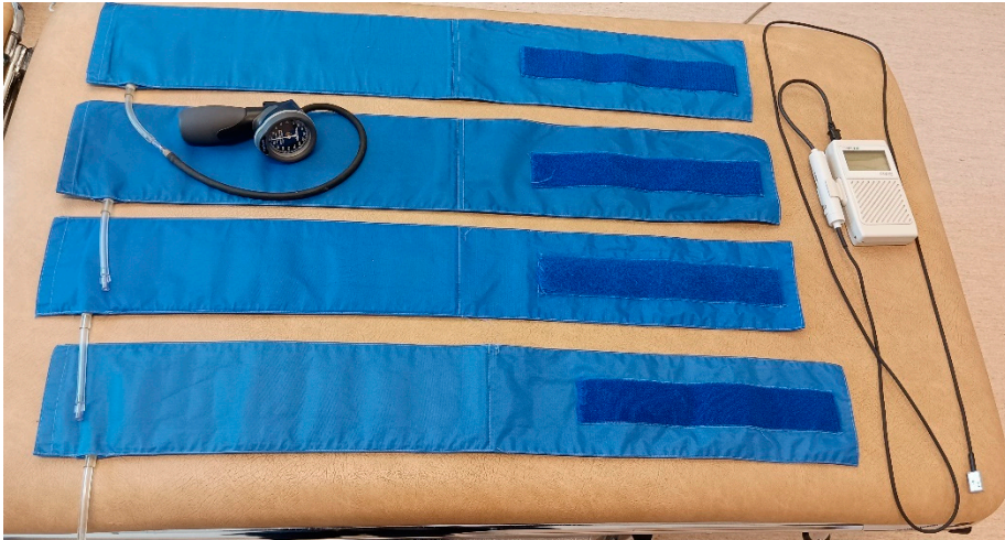
Figure 8. Four pressure cuffs for 2 arms and foot ankles with the sensor used in MOS ( Shantanu Sharma ).
