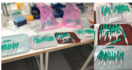
Figure 11c. Step 3) Prepare the syringes and labelling. Cream preparations are filled in 2-ml plastic syringes. The syringes are labelled and stored at +4°C.
