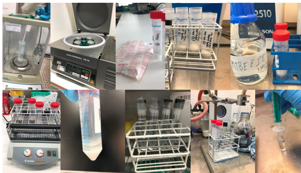
Figure 12. Preparing the repeated open application test creams for chemical analysis by using gas chromatography-mass spectrometry.
