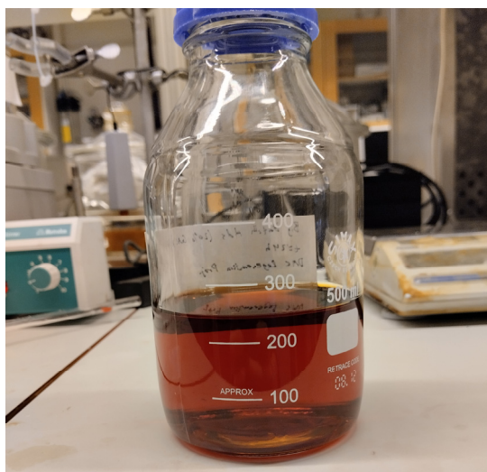
Figure 6.7. The 250 mL purified HMF batch from the adsorption process, to be evaporated.
