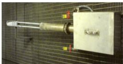
g. IACM mirror probe used when only one access port is available
