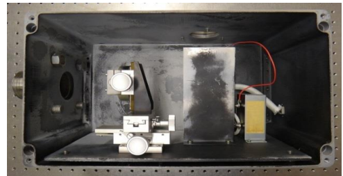
b. The IACM transmitter with xenon lamp and collimating lens.
