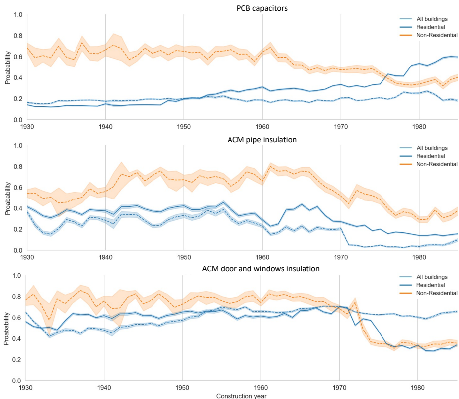
Figure 3.9. Predicted probability distribution of selected asbestos and PCB materials along the construction year by all buildings (in continuous line) and building categories (in dashed line), as detailed in Paper IV.
