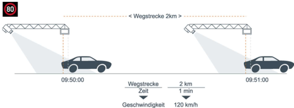
Figure 21. Section speed control (Stefan, 2006).
