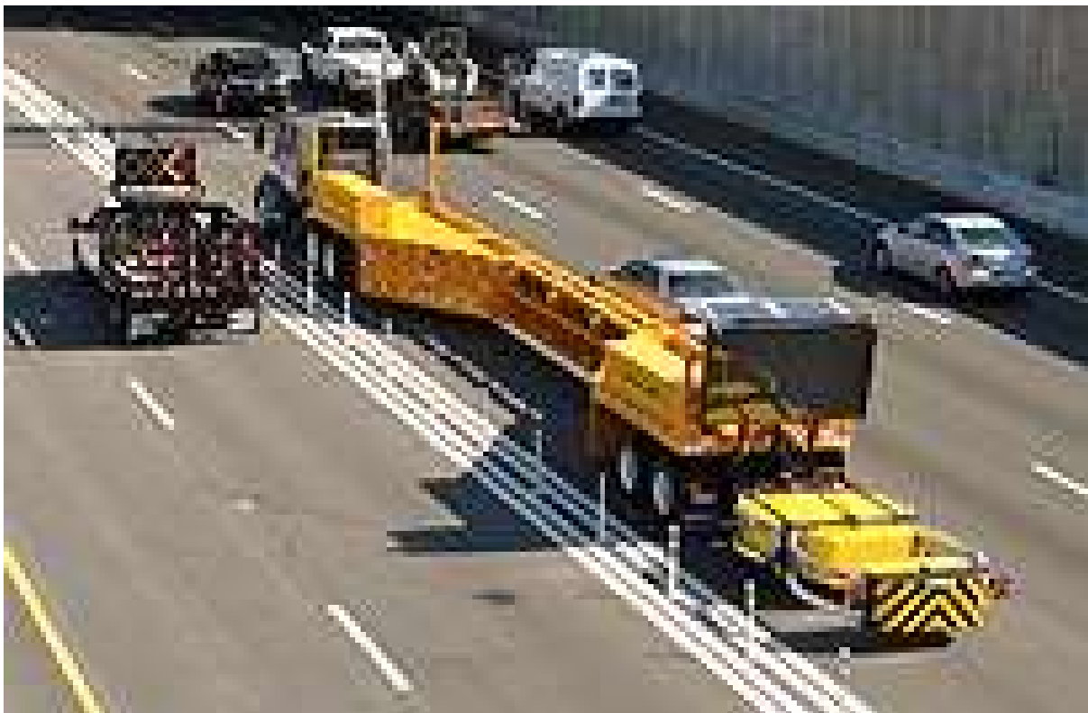
Figure 23. Mobile Barrier Trailer MBT-1. http://www.barriersintl.com/mobilebarriers/images/Photos/day/Mobile%20Barriers%20MBT-1%20Capital%20Beltway%20I-495%20Express%20Lanes/vertical/tb-Mobile%20Barriers%20MBT-1%20Capital%20Beltway%20I-495%20Express%20Lanes%20Maintenance%205.JPG
