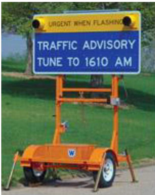
Figure 5. Highway Advisory Radio System (HAR). ( https://www.google.se/search?q=Highway+Advisory+Radio+Systems&dcr=0&tbm=isch&source=iu&ictx=1&fir=NztKHIMwMMnP3M%253A%252CSUucky9z00lo6M%252C_&usg=__gqBMM_hZZrfKAxZKFSTe8hPjPhA%3D&sa=X&ved=0ahUKEwi43tOi7pPZAUBZCwKHUQhCBsQ9QEIQjAG#imgrc=P9PI4uXo6EfWnM: )
