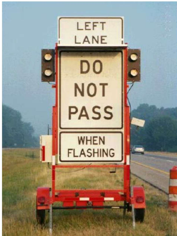
Figure 9. Dynamic lane merger sign (Bushman et al., 2003).
