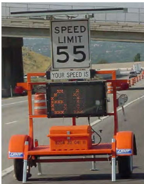
Figure 13. Speed Monitoring Display (Bowie, 2003).
