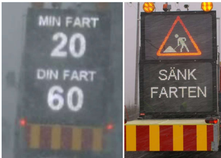
Figure 15. TMA with two Variable Message Signs (text in Swedish). Alternative C with the two phases: 1) "MIN FART" ("MY SPEED") and "DIN FART" (YOUR SPEED"; 2) road work warning sign and "SÄNK FARTEN" ("REDUCE SPEED" (Sørensen & Wiklund, 2010).
