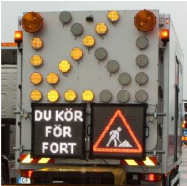
Figure 14. VMS with the text "You drive too fast" (in Swedish) if the driver drove faster than the recommended speed on TMA. " (Sørensen & Wiklund, 2010).
