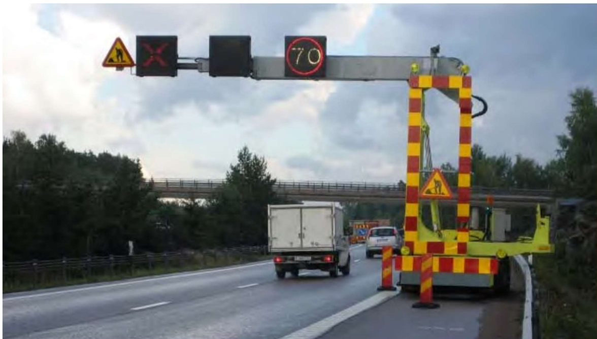
Figure 1. A mobile gantry crane for quick setup of signs at newly established road work zone (Bolling & Sørensen, 2008).
