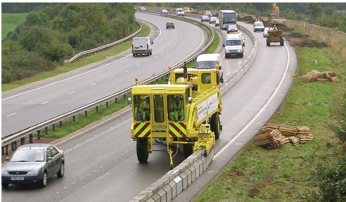
Figure 23. A “Quick moveable barrier” ( http://www.barriersystemsinc.com/stuff/contentmgr/files/0/06bcc8d5b07bf7de9c026797c585635/files/qmb_const_pi_sheet_international_04_18_13.pdf )
