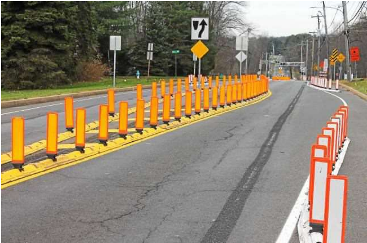
Figure 18. A chicane ( http://www.buckslocalnews.com/news/yardley_area/engineer-updates-lower-makefield-supervisors-on-sandy-run-road-engineering/article_2c447361-1858-58c5-bb6c-3b252b1bae37.html ).
