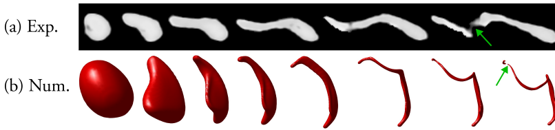
Figure 4.9: Single-point breakup morphology for (a) Experimental drop, and (b) Numerical drop. The green arrows show the initial breakup point.
