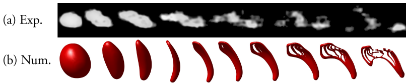
Figure 4.10: Diffuse breakup morphology for (a) Experimental drop, and (b) Numerical drop
