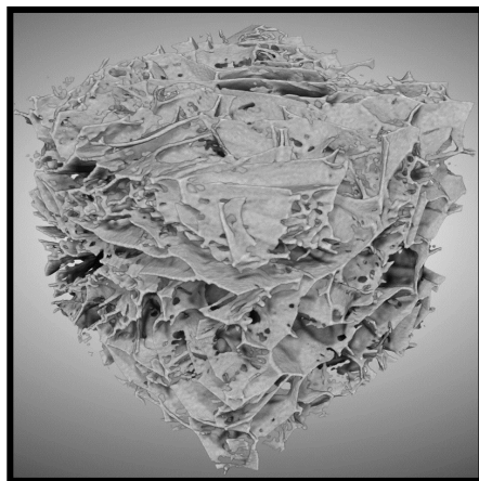
Figure 14: Tomographic 3D image of 10% maltodextrin freeze-dried in vial. The 3D-rendered image can be used to quantify material properties.
