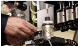
Figure 1. The sample environment under installation at ForMAX
