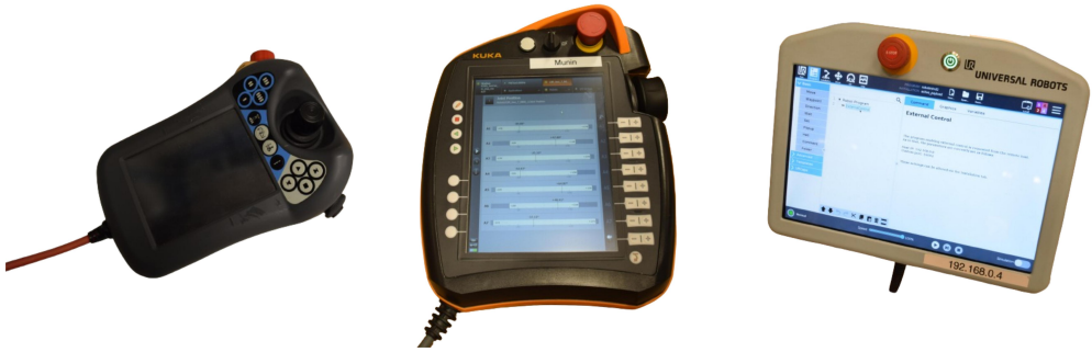
Figure 2: The teaching pendants of three different robot manufacturers. From left to right: ABB , KUKA and Universal Robots (UR) .
