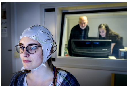
Figure 3.6 EEG recording device. The electrodes are placed on a cap that the user wears on the head.
