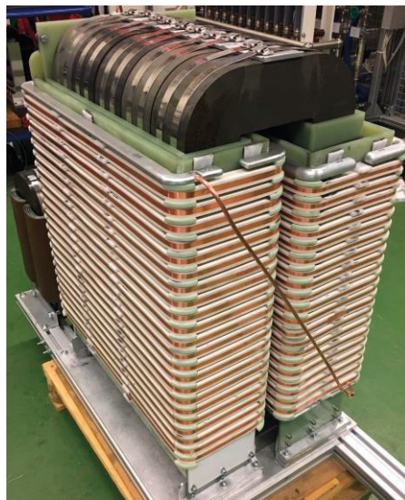
Figure 4.90: Pulse transformer unit used in commercial modulator (after refurbishment of secondary windings)
