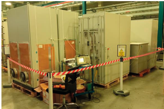
Figure 9.3: Overview of prototype converter chain including high-voltage oil tank assembly and load cabinets. Three resistive load cabinets are obscured by the low-voltage cabinet.
