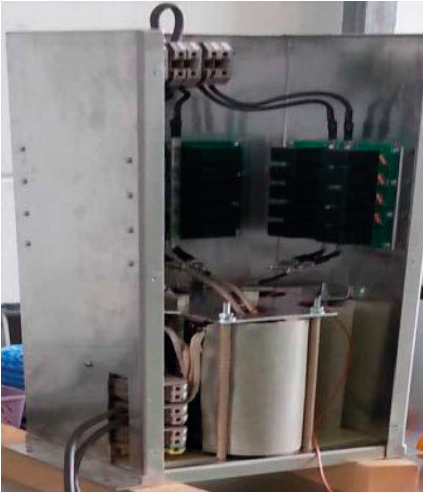
Figure 8.6: Developed common mode filter assembly
