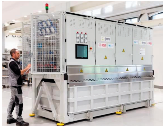
Figure 9.1: Overview of complete SML modulator developed for ESS klystron requirements
