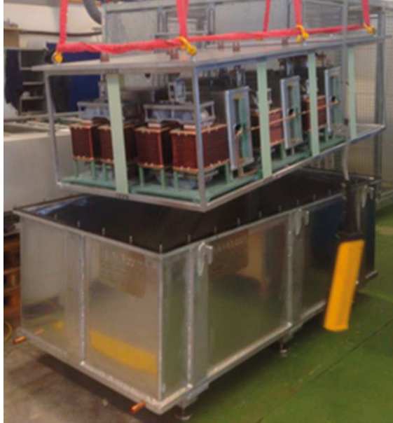
Figure 8.10: High-voltage assembly being lowered into oil tank
