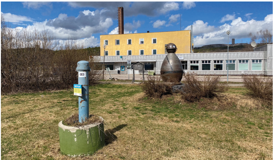
Figure 10. A monument called the mining-oldster ( gruvgubbe ). In the foreground a stick that measures vibrations during explosions in the mine. They are placed throughout MalMBERGET and Kiruna and measure dangerous levels of vibration in proximity to housing and public spaces. (O7)
