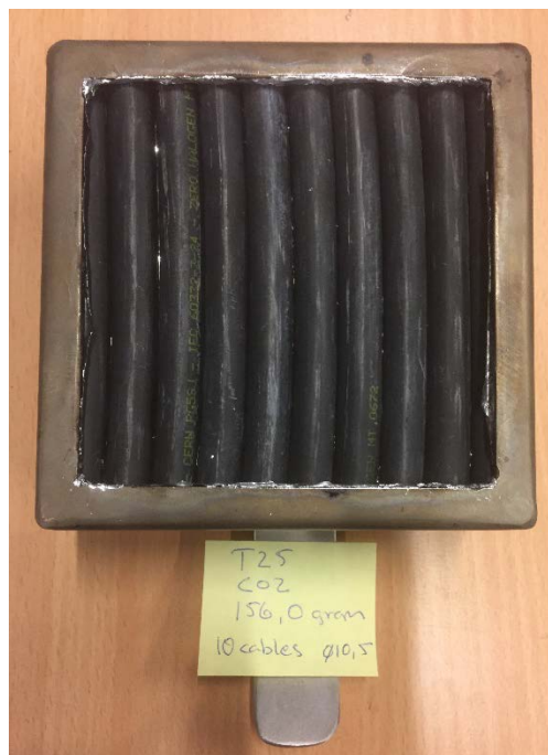
Figure 2. Example of cables in sample holder prior to test.
