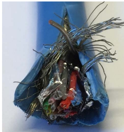
Figure 4. The cables consist of a sheath, metallic shielding and the conductor(s) with insulating material.
