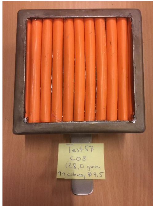
Figure 4. Example of cables in sample holder prior to test.
