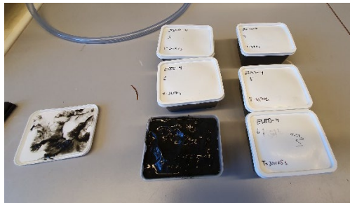
Figure 14 Sediment samples prior to drying (left) and after drying (right).
