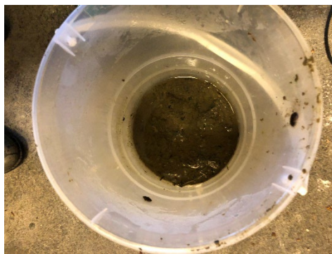
Figure 5 The bucket in the lower right photo in Figure 4 after 1.5 days of sedimentation. Clear water is above the sediment at the bottom of the bucket.
