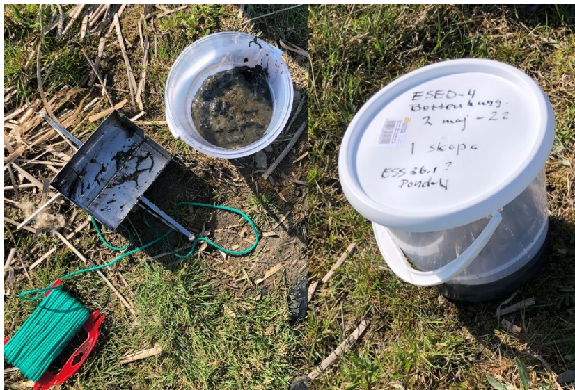
Figure 11 Sediment sample collected with the Lamotte bottom sampling dredge, 2 May 2022.
