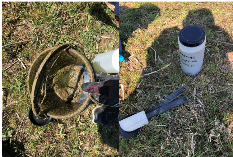
Figure 7 ESED_3:31:6 collected between 16 September 2021 and 2 May 2022. The plastic spoon and scraper were used to transfer the sediment from the 5-L bucket to the 2-L container.
