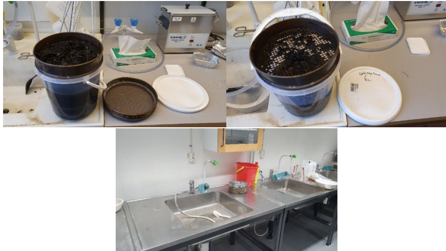
Figure 13 Sieving of sediment samples. The two upper photos demonstrate the sieving procedure. The bottom photo shows the sinks with sediment traps at the sediment lab at the Department of Geology, Lund University.
