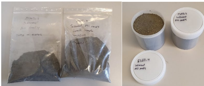
Figure 16 Left: Homogenized, dried, and homogenized sediment samples. Right: 200-mL sample jars with dried and homogenized sediment samples for gamma-ray spectrometry.
