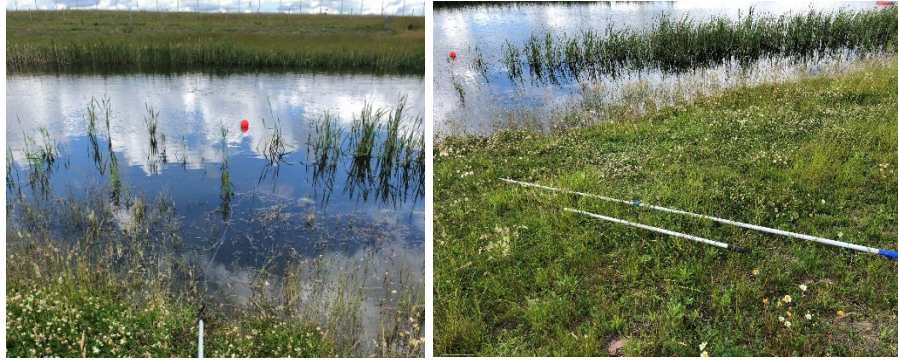
Figure 3 Pond at the ESS (site 31.6, N55.74, E13.24), 22 June 2020, including boathooks (one of length 1.7 m and one telescopic of length > 4 m) and marker float for the bottom sediment sampling trap.
