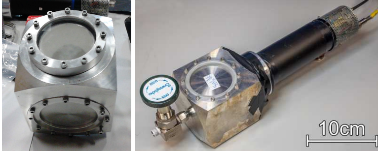
Figure 2: Fission-fragment detector. Left panel: photograph of the ^4\text{He} gas cell. Right panel: photograph of the gas cell and PMT assembly. The PMT assembly is the black cylinder to the right. (For interpretation of the references to color in this figure caption, the reader is referred to the web version of this article.)
