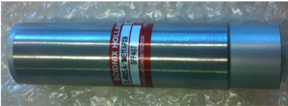
Figure 2.3: Photograph of a YAP detector. The PMT and the PMT assembly (base and magnetic shielding) are located on the polished side to the left. The YAP crystal is located under the matt surface to the right.
