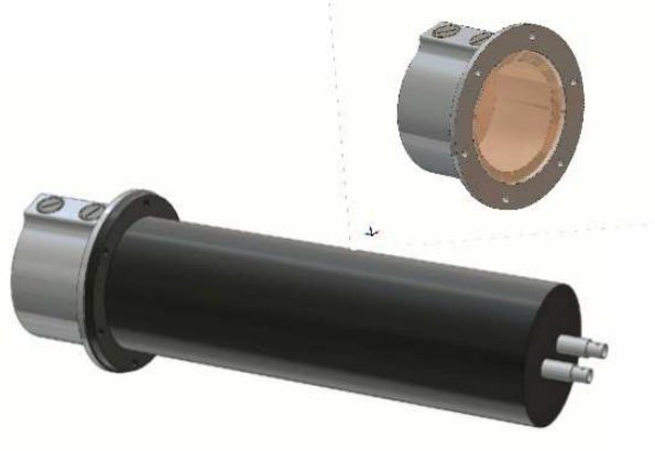
Figure 4: The NE-213 detector (CAD representation). Top: the aluminum scintillator “cup”. A borosilicate-glass window (light brown) separates the scintillator and lightguide. Bottom: The “cup” is to the left. The \mu -metal shielded PMT and base assembly is the black cylinder to the right. Figure from Ref. [18]. (For interpretation of the references to color in this figure caption, the reader is referred to the web version of this article.)
