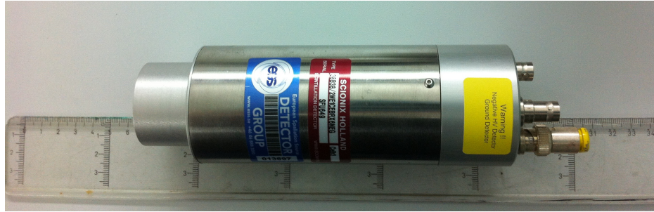
Figure 2.4: Photograph of the \text{CeBr}_3 detector. The scintillator crystal is to the left. The PMT and the base are to the right.
