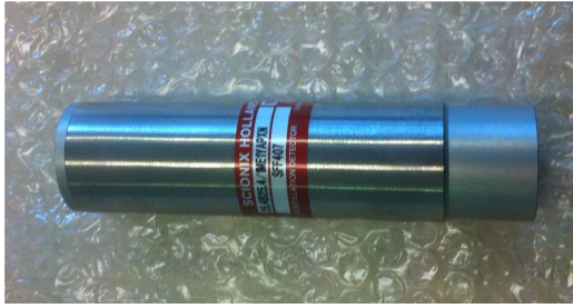
Fig. 2. Photograph of a YAP(Ce) detector. A cylindrical 1 in. long by 1 in. in diameter crystal (right) was coupled to 1 in. diameter PMT. Figure from Ref. [7].
