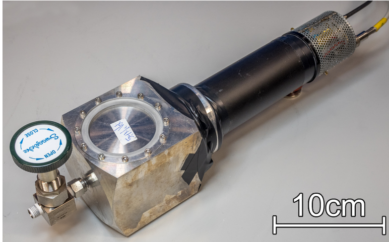
Figure 2.7: A picture of the ^4\text{He} fission fragment detector. From left to right, a high pressure valve, the aluminum pressure vessel and the PMT assembly with a black mu-metal shield are shown.
