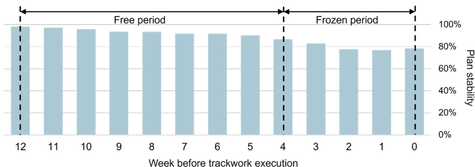
Figure 12. Trackwork plan stability estimate for each week in the rolling horizon plan (Paper 3).
