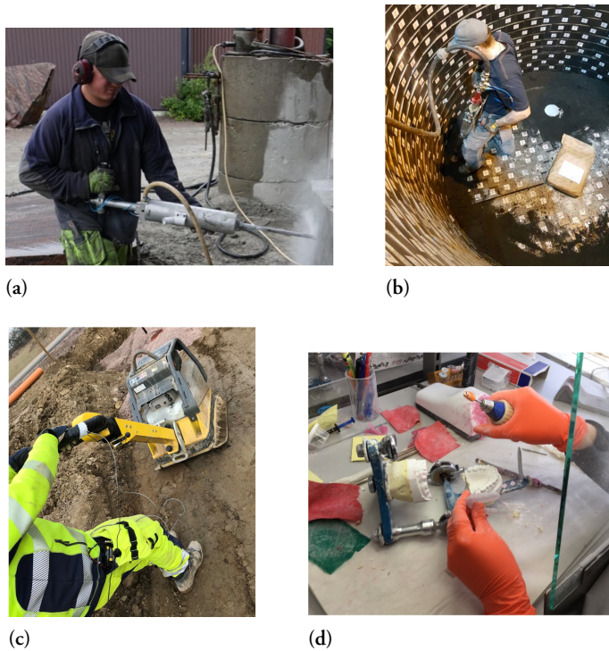
Figure 4: The different tools for which low-vibration prototypes were developed within the four industries. The figure shows the rock drill (a), the rammer (b), a vibration plate (c) and a dental hand-piece (d).
