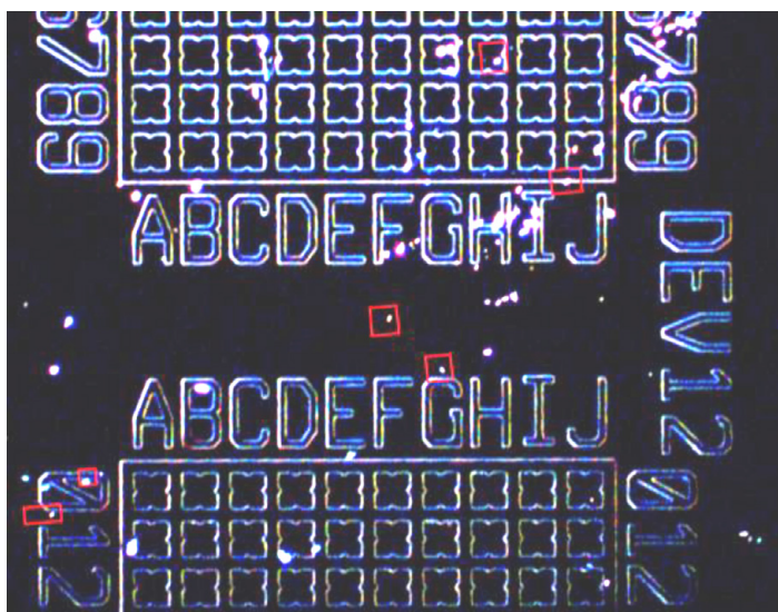
Figure 3.12: A gold-covered Si substrate with a pattern enabling the identification of single NWs. Single NWs are indicated on the substrate by red rectangles.
