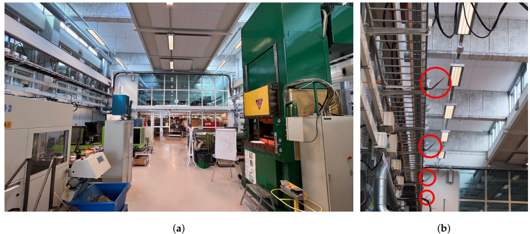
Figure 5. (a) A photograph showing a view of the environment. The hall is approximately 30\text{ m} \times 11\text{ m} with a ceiling height between 8 m to 10 m depending on location. (b) A photograph showing the placement of four antennas (circled in red). In total, there were twelve distributed antennas; six on each side of the hall. They were situated 4 m above the floor, with a separation of 4 m.
