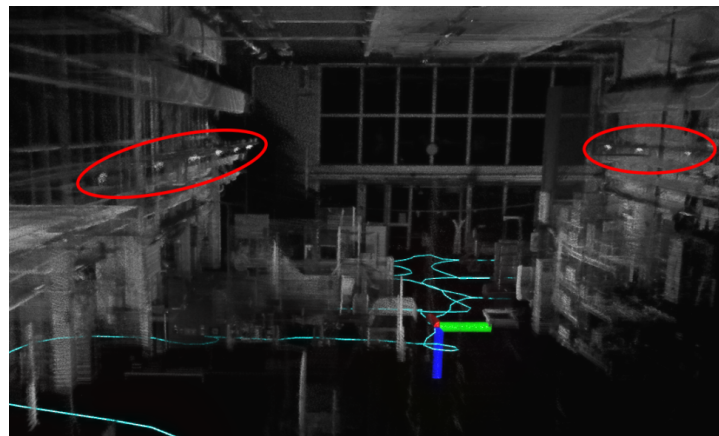
Figure 6. Example output from FAST-LIO2 . The figure depicts the intensity of the points in the scan, and the extra intensity spots on antenna locations with the help of reflective tape, as seen in the circled regions. The cyan colored path shown is an example output of the ground truth position of the user.
