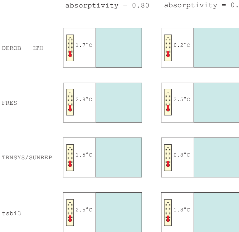
Figure 4.55 Mean temperature for the winter day. The solar gains are based on the four programs.
