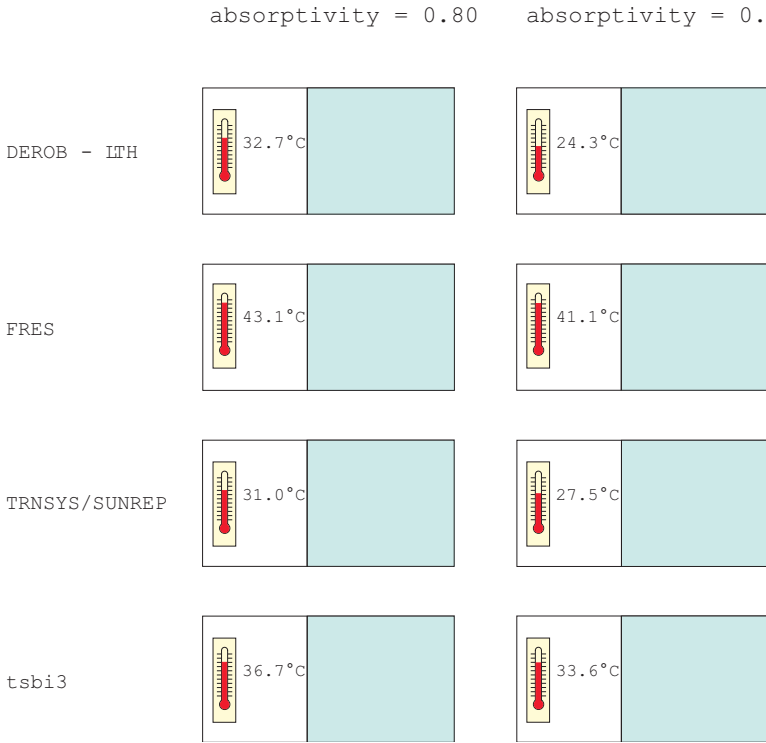
Figure 4.57 Mean temperature for the summer day. The solar gains are based on the four programs.
