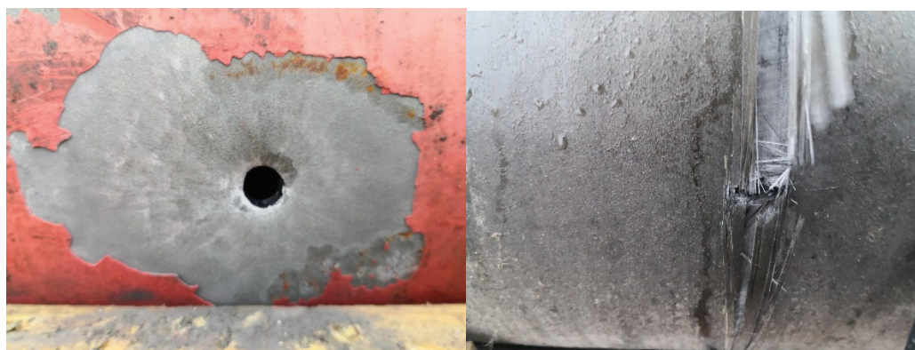
Figure 5. Typical holes from penetration with rifles in type I (left) and type III and IV (right) vessels
