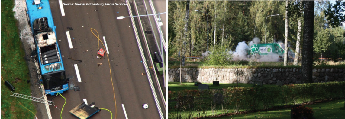
Figure 1. (Left) Picture from the bus fire where two firefighters were injured after vessel rupture in Gothenburg in 2016. (Right) Picture from the garbage truck accident where a rifle was used for depressurization, at the moment of tank rupture.
