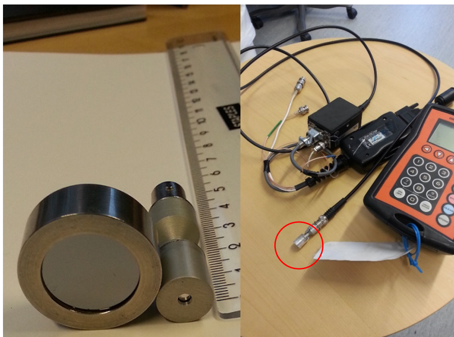
Figure 1. A 300 mm 2 ion implanted silicon detector (ISD) next to the 4 mm 2 Si CT dose profiler (CTDP), here without aluminum Mylar foil. The CTDP is contained within a cylinder with a 2.5 mm (Ø) aperture (left picture). The CTDP, indicated by a circle, connected to a charge-sensitive preamplifier (2003BT) and a digital portable multichannel analyzer (DigiDart™) (right picture).
