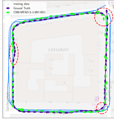
Fig. 11. Predictions and ground truth for the MFAD representation CNN-MFAD-S-3.8M HEU overlaid on a map for the high epistemic uncertainty case. Note that the network does not tend to project to places outside the training set (emphasized with dashed red ellipses).
