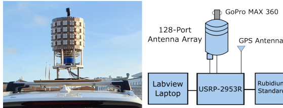
Fig. 3. Picture and block diagram of LTE measurement system. A GoPro MAX panoramic camera was used to capture video of the environment as seen by the antenna array, and an OXTS 3003G system was used for ground truth pose estimates. All systems held time synchronization with GPS Time as a time base.
