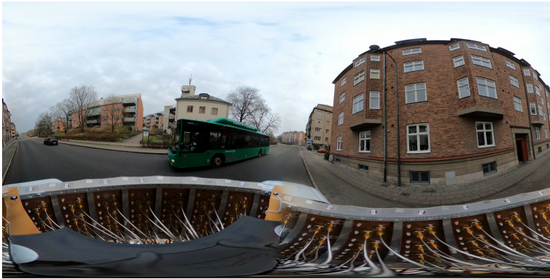
Figure A.3: Panorama image showing the view from the GoPRO camera, mounted on top of the antenna array. The SMA connections to the upper rows of patch antennas are visible in the lower part of the image, and the base station is visible above the bus.
