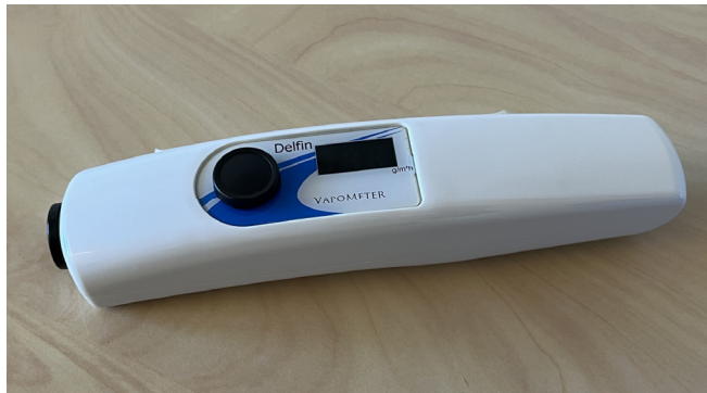
Figure 12. The closed chamber TEWL meter, the Vapometer 300 (Delfin Technologies Ltd, Kuopio, Finland). Photo: Emma Belfrage
