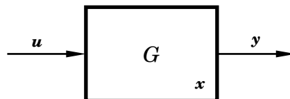
Figure 1.5 Graphical block representation of a dynamical system G with input signal \mathbf{u} , output or measurement signal \mathbf{y} , and internal state \mathbf{x} . The arrows indicate signal flow directions.
