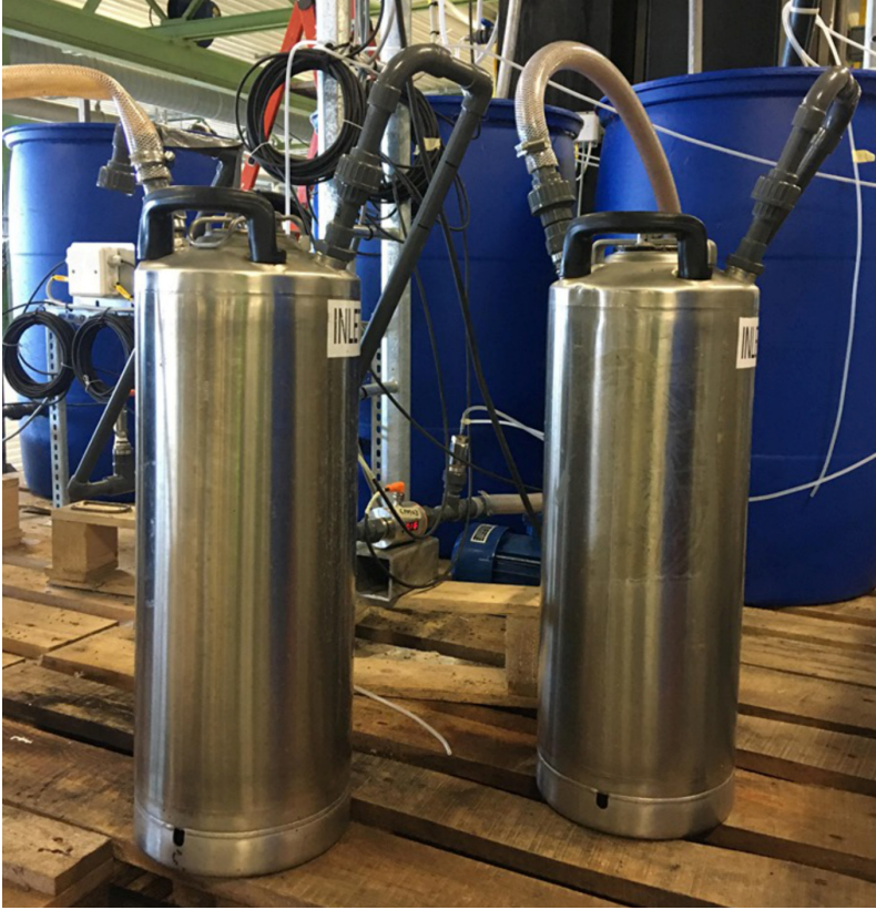
Figure 10. Photograph of pilot-scale GAC (left) and sand (right) filter at Svedala WWTP. Photograph by Alexander Betsholtz and Simon Gidstedt.
