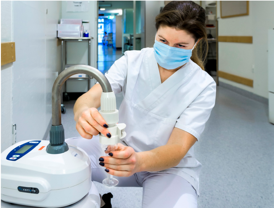
Figure 4. The Coriolis \mu liquid cyclone operated in a hospital corridor. Photo by Kennet Ruona
