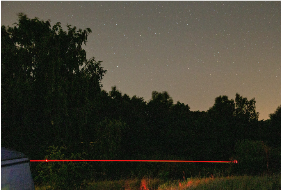
Figure 3.10. The elastic hyperspectral lidar (EHS�) at Stensoffa field station, Sweden, measuring wing thicknesses of insects remotely. A flash in the laser beam indicates an illuminated insect. This work is included in Paper III. Image attribution iv .
