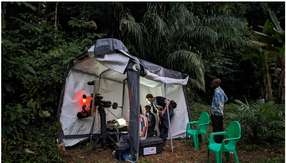
Figure 2.6. Meng, Adolphe, Doria, Mikkel, and Benoit by the lidar, conducting remote sensing of insects in Tai rainforest, Côte d'Ivoire, as part of Paper VI. The motorized tripod was programmed to sweep to different angles, so different heights of the canopy were probed.
