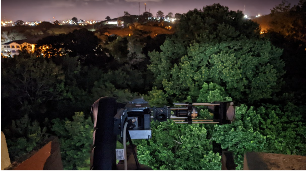
Figure 2.4. A remote fluorescence measurement of a tree canopy at the campus of the University of Cape Coast, Ghana. The canopy structure was scanned at the same time as fluorescence measurements from the leaves were acquired as part of Paper VIII.
