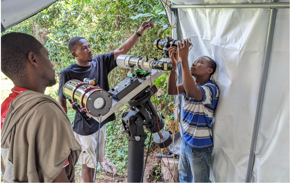
Figure 4.11. Andrew, Rabbi, and Adolphe are aligning the Scheimpflug lidar in a virgin rainforest in Côte d’Ivoire for measuring insect biodiversity (Paper VI). Left to right on the baseline there is mounted a receiving Newton telescope, a laser driver box, a monitor camera telescope, and a laser expander with two laser diodes.
