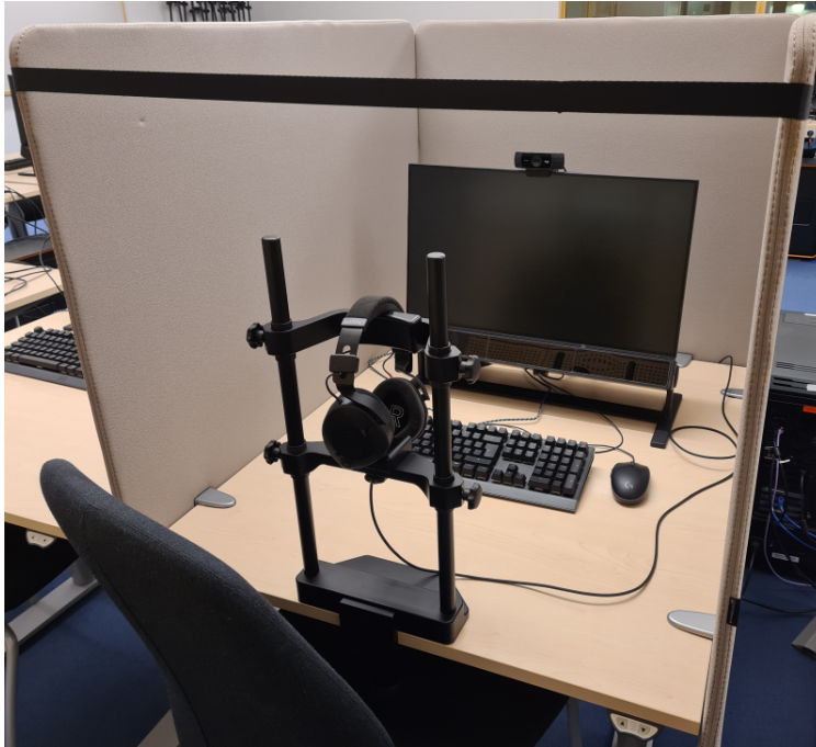
Figure 1: A video-based eye tracker attached to the bottom of a monitor with a chin rest.
