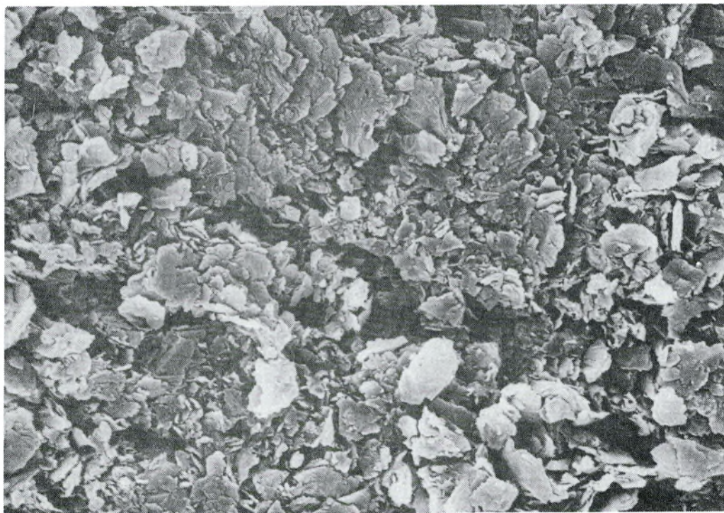
Fig. 6. Scanning electron microscopy pictures showing the surface of a graphite electrode polished on fine emery paper. Magnifications (a) x500 and (b) x1500.
