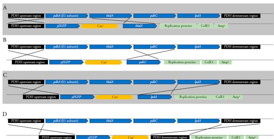
Figure 7: Schematic representation of the attempted double-crossover integration. (Black = PDH operon upstream and downstream regions; Blue = the genes in the PDH operon; Yellow = selection pressure with Cre-LoxP sites; Green = pNZ5319 backbone)
