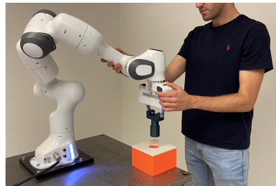
A human operator manually guiding a robot to teach a peg-in-hole task.
