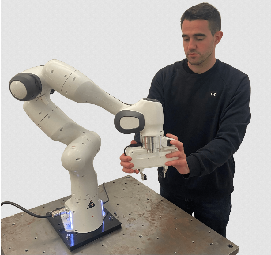
Figure 3. A human–robot collaborative scenario where an operator was guiding a Franka Emika Panda robot mounted on a table.
