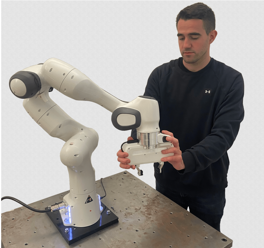
Figure 3.4 A human–robot collaborative scenario where an operator was guiding a Franka Emika Panda robot mounted on a table (figure included in Paper VI [Salt Ducaju et al. , 2024b]).
