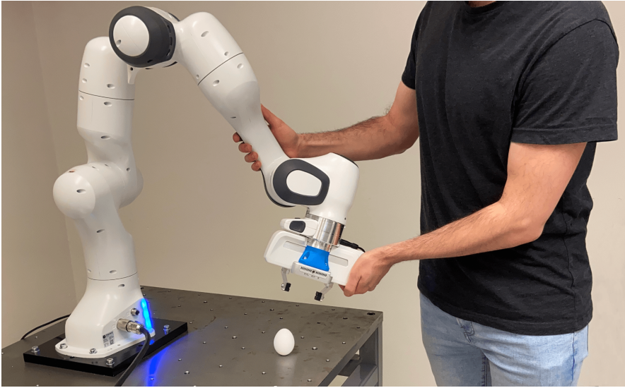
Figure 1. Setup for the kinesthetic teaching task described in Sec. 4.2. A Franka Emika Panda robot is mounted on a table. The blue piece allows to attach a camera to the robot’s end effector. The human operator is manually guiding the robot and displacing it away from its original trajectory and arbitrarily close to the object of interest, here, an egg.
