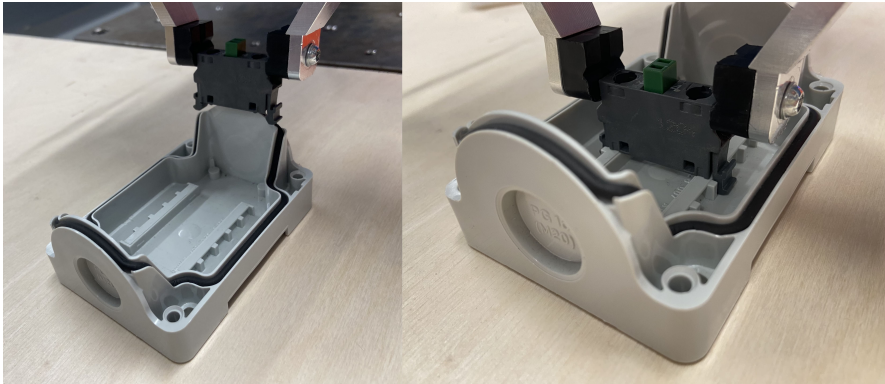
Figure 9. Comparison between the final position of the switch before iterative learning was used (left) and after eight iterations of the proposed learning controller (right) for the snap-fit assembly of a switch.
